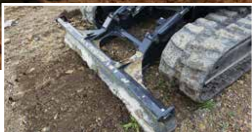
The floating blade feature is standard for the product range, allowing each operator a perfect levelling result.
