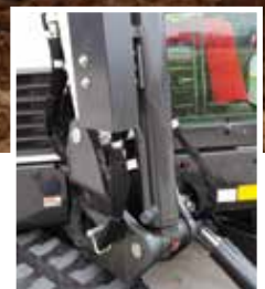
Standard boom and arm safety valves to guarantee safety at all times
