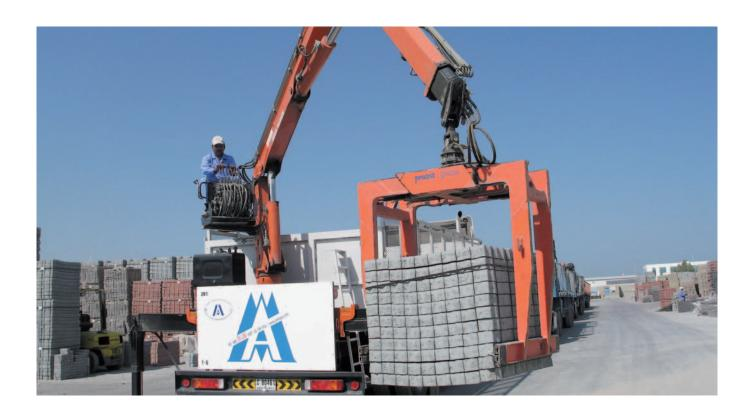
We have developed various types of Block Loading Grabs specially equipped for your needs and loads:
