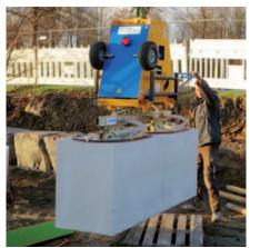
producing a significantly faster buildup of vacuum, also suitable for more porous elements. Complete automatic drive via integral petrol engine with electric starter.
