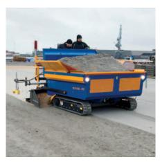
Sideways foldable chutes to avoid that material is spilling over the side of the hopper.
