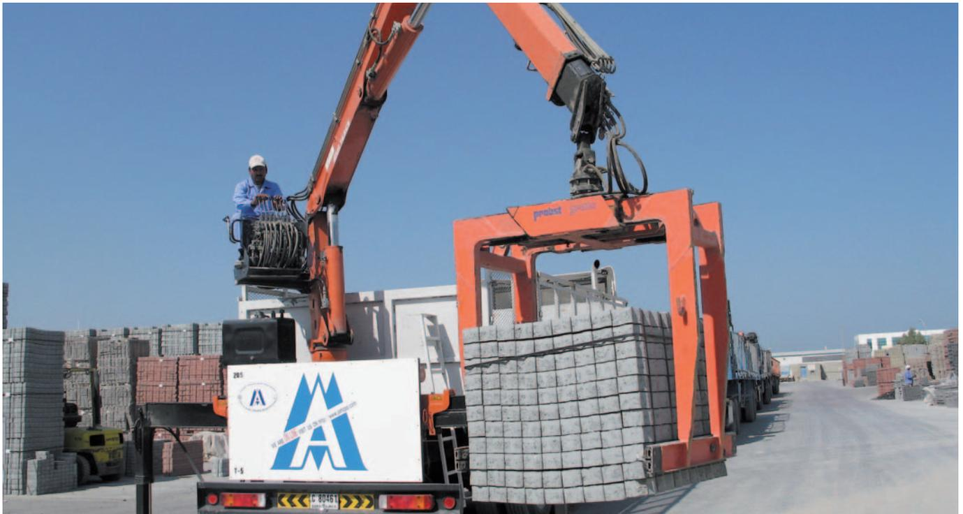
We have developed various types of Block Loading Grabs specially equipped for your needs and loads:
